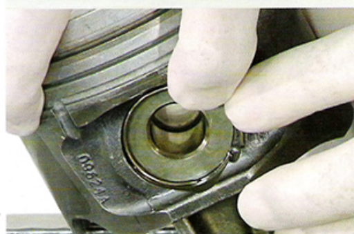
Fig.4 - Inserindo as travas
