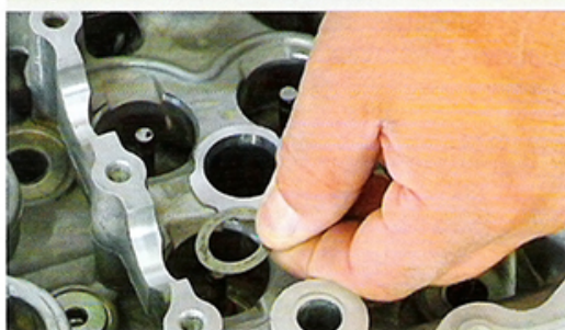
Fig.4 - Colocando as arruelas
